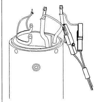
Replacing excitation winding
